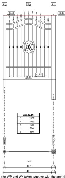
LEGEND: S(So) – element width [mm]; H – element height [mm]; a – upper crossbar position (for WP and Wk taken together with the arch) [mm]; b – lower crossbar position [mm]; c – arch height [mm]
