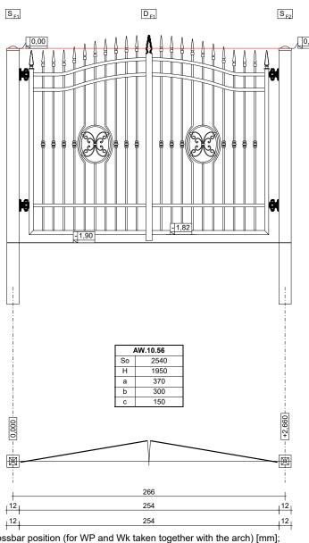
LEGEND: S(So) – element width [mm]; H – element height [mm]; a – upper crossbar position (for WP and Wk taken together with the arch) [mm]; b – lower crossbar position [mm]; c – arch height [mm]
