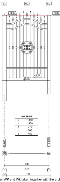
LEGEND: S(So) - element width [mm]; H - element height [mm]; a - upper crossbar position (for WP and Wk taken together with the arch) [mm]; b – lower crossbar position [mm]; c – arch height [mm]
