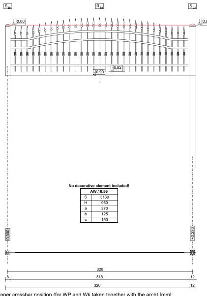
LEGEND: S(So) – element width [mm]; H – element height [mm]; a – upper crossbar position (for WP and Wk taken together with the arch) [mm]; b – lower crossbar position [mm]; c – arch height [mm]
